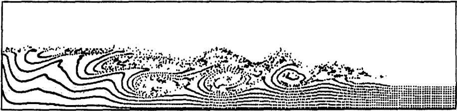
FIG. 3. Bore at R = 79.25 showing large eddy structure. Configuration shown at t = 11.00 .
